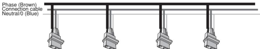
To ensure you know the smoke detectors are inactive in case of power failure, ensure a vital part of your lighting is attached to the same power group. Please view national standards for proper installation procedure.
